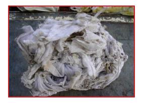
Mounds of wipes removed from a clogged pump at the Willow Brook Pump Station, New Britain.
